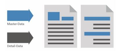
Effect of the option AutoMasterMode. Left: "AsVariables", right: "AsFields".
